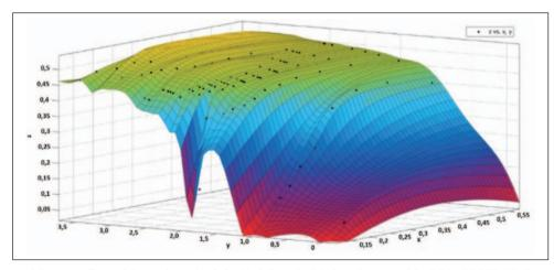
**Fig. 6** Three-dimensional Form  $\eta_i = f(\alpha, q_{cvcl})$  Dependence Made by Modelling the Working Process of the DE by BOOST AVL (here:  $x - q_{cvcl}, z - \eta_i; y - \alpha$ )
