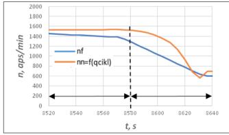
Fig. 10 Change in the CAT3512B-HD DE Energy Efficiency Parameters in the Process of Slow Acceleration
