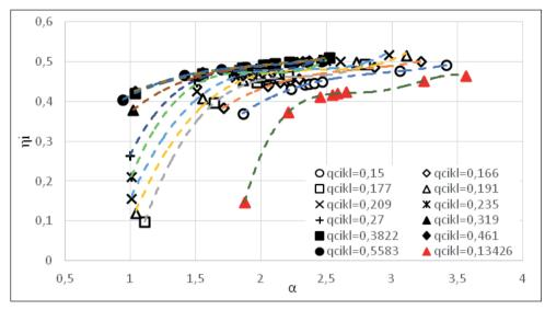
Fig. 5 Two-dimensional Form  $\eta_i = f(\alpha, q_{cycl})$  Dependence, Obtained by Modelling the Process of the DE Working Process in BOOST AVL
