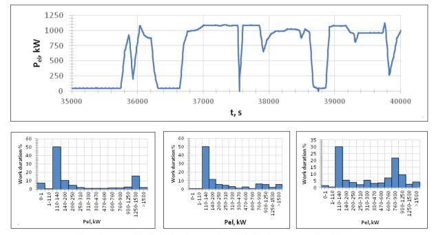
Fig. 1 Structure of the Cycle of an Operational Load of a Freight Locomotive Diesel Engine:
